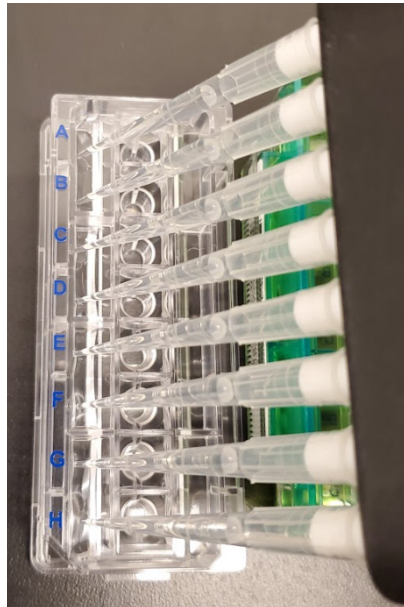
Figure 5. An 8-channel P200 pipettor is used to fill the cartridge moats.
