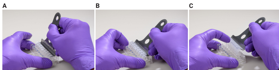
Figure 6. (A) insert the prongs of the removal tool between each well, keeping the bottom of the tool parallel to the top of the plate. (B) once the prongs are inserted, lever the mask from the wells of the plate. (C) Hold the mask onto the removal tool with one finger as its being lifted from the plate to prevent it from falling.
